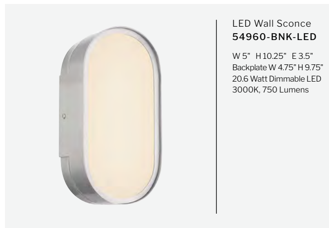
LED Wall Sconce 54960-SB-LED W 5" H 10.25" E 3.5" Backplate W 4.75" H 9.75" 20.6 Watt Dimmable LED 3000K, 750 Lumens
