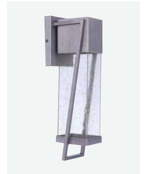
Medium LED Wall Mount ZA4414-BT-LED WET RATED W 4.75" H 17" E 5.75" Backplate: W 4.75" H 6" 15.44 Watt Dimmable LED 3000K, 536.4 Lumens
